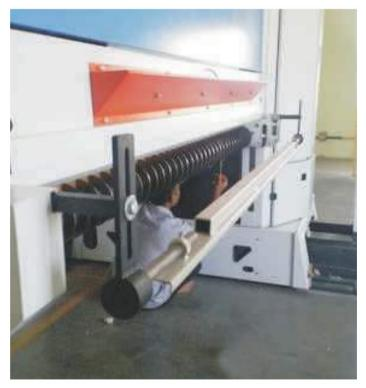
We Offer Blendomat / Bale Plucker Magnet mainly used for removing the Heavy Metal particles from the Bales. Most of the Fire causes due to Metal and Bale Plucker / Blendomat Beater get contact. To avoid the huge loss from Cotton and Machineries Fire accident, install our Magnet in the Bale Plucker / Blendomat Machine.
